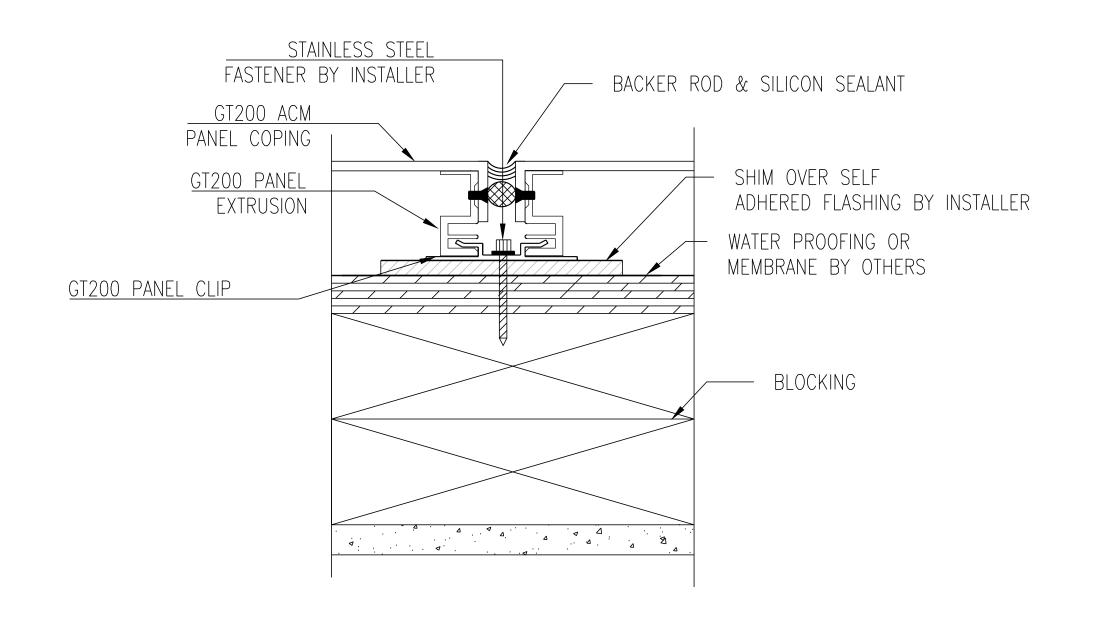
COPING PANEL JOINT DETAIL SCALE: NTS
